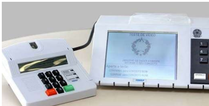
Figure 1. Brazilian voting machine and its two terminals. The election officer terminal is on the left and the voter terminal is on the right.
